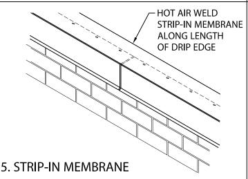
HOT AIR WELD STRIP-IN MEMBRANE ALONG ENTIRE LENGTH OF DRIP EDGE PER MANUFACTURERS INSTRUCTIONS.
